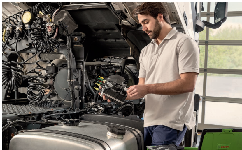
Replacing a Bosch supply module on a truck
